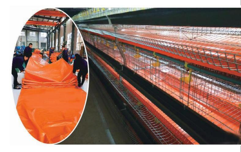
PVC conveyor belt material, also known as removal belts, is used to make various conveyor belts for applications in machinery, agricultural equipment, livestock farming, factories, food processing, and automation systems. The material is highly flexible, easy to assemble and disassemble, and occurries minimal space.
